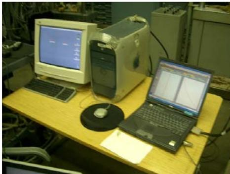
Figure 7. Picture of the Mac computer used to run the controlled strain loading and unloading cycles and to collect data for plain concrete beam tests, and laptop used to collect all the data for a FRC beam test.
