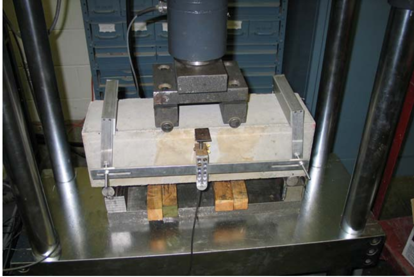
Figure 2. Fiber-reinforced concrete beam before testing.
