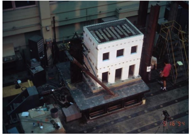
2-story Unreinforced Masonry Building.
