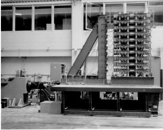
Seismic Tests of 10-story RC Frame-wall Building as part of Abrams' doctoral dissertation.
