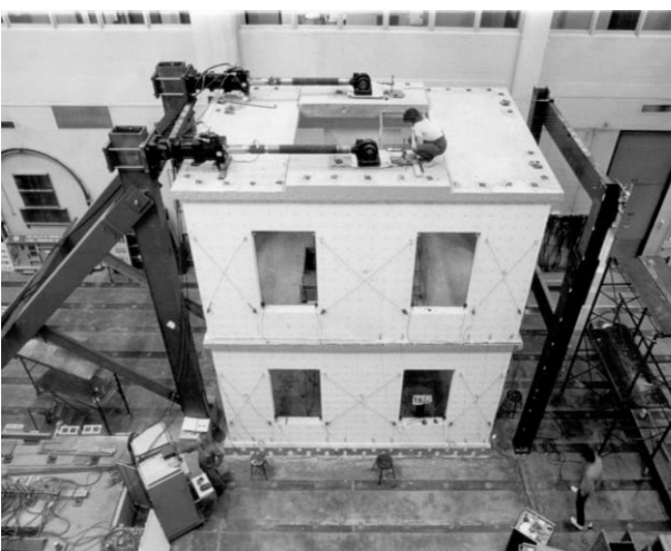
2-story Full-Scale Reinforced Masonry Building.
