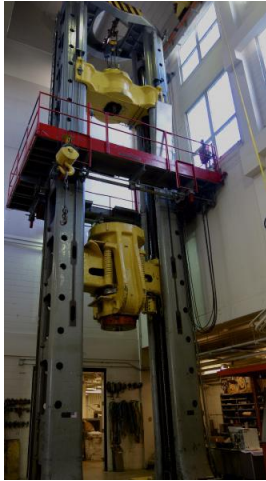
3,000 kip (13 MN) Testing Frame built in 1929
