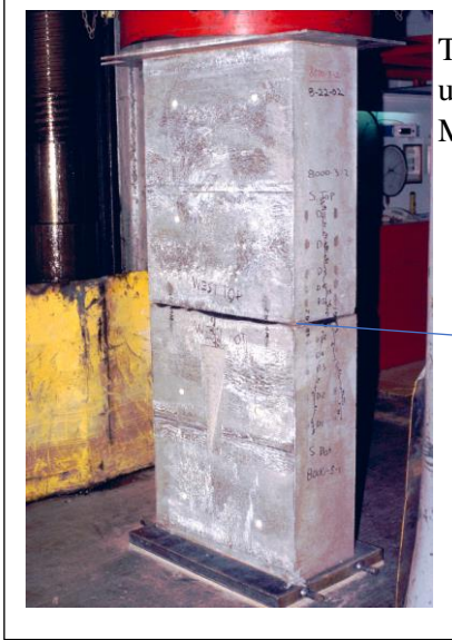
Tunnel liner tested using 3,000 kip (13 MN) Testing Frame.
