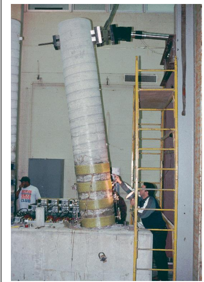
Testing the concrete column retrofitted with fiber glass.
